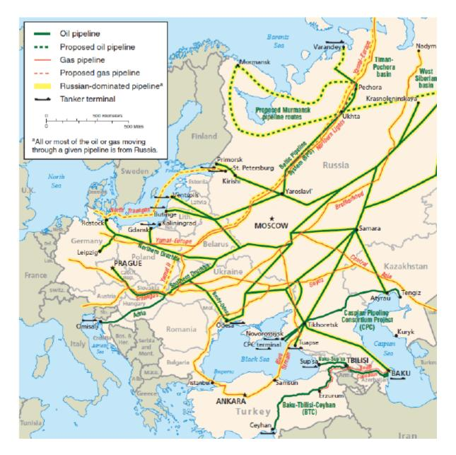
Map of Russian Oil and Gas Pipelines Feeding Europe (Source: US Energy Information Administration. "Map of oil and gas pipelines from Russia." – Research Gate, Uploaded by Juraj Kubica, Published 2019 on <a href="https://www.researchgate.net/figure/Map-of-oil-and-gas-pipelines-from-Russia-credit-US-Energy-Information-Administration fig2 268047847">https://www.researchgate.net/figure/Map-of-oil-and-gas-pipelines-from-Russia-credit-US-Energy-Information-Administration fig2 268047847</a>)
